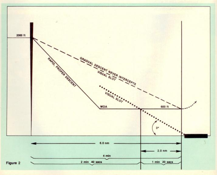
Conversely, failure to consider the effects of a headwind could result in flying an abbreviated final approach course. During conditions of minimum visibility, this would require having to execute a pullup before getting close enough to the airport to establish visual contact.
